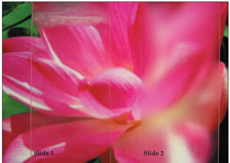
Fig. 1 — Slide 1 is a piece of glass coated with silica nanoparticles. Slide 2 is an uncoated piece of glass. MIT Professors Cohen and Rubner have discovered that thin film coatings comprised of nanoparticles of glass that are about one million times smaller than a grain of sand interact so strongly with water that they force the condensing water droplets to spread out into an ultrathin sheet of water in a fraction of a second.
