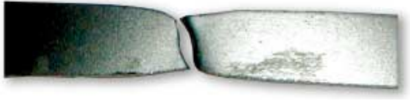
This tensile specimen has been pulled to fracture and depicts the region where necking occurred. Graphic: ADMET Inc.
