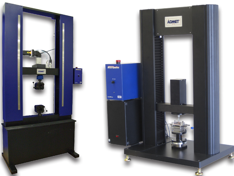
ADMET eXpert 3600 Floor-Standing (L) and Table Top (R) Axial-Torsion Test Systems
