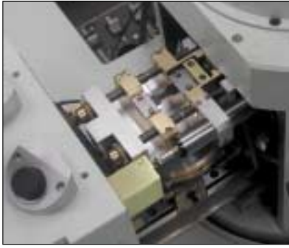
Fig. 2 — A 5 kN-capacity palm-sized tensile stage mounted inside a Scanning Electron Microscope (SEM). Picture shows a dog bone-shaped polymer specimen clamped in the stage. Tensile stage manufactured by Ernest F. Fullam Inc., Latham, New York.
