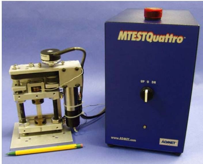
Micro EP 5kN Tensile Stage equipped with ADMET's MTESTQuattro™ Materials Testing System
