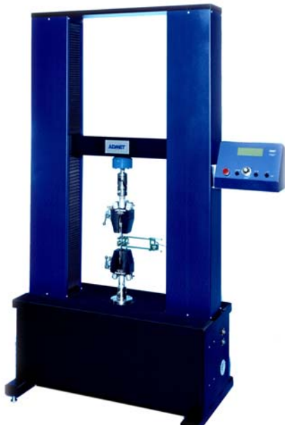
ADMET eXpert 2653 universal test frame
