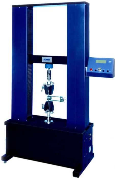
ADMET eXpert 2653 universal test frame
