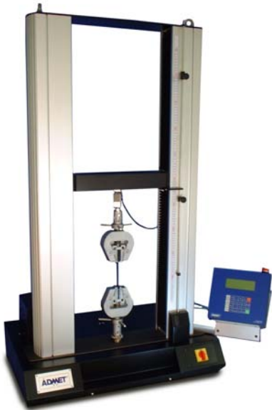
ADMET eXpert 2611 universal test frame
