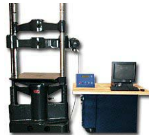
60K Baldwin upgraded with new servo-hydraulic power unit and ADMET's MTESTQuattro Materials Testing System.
