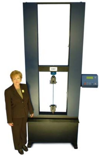
eXpert 2653 modified for 24 inches of additional crosshead travel.
