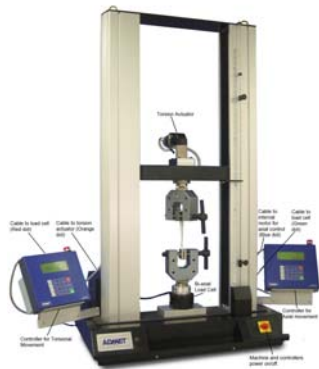
eXpert 2610 5kN with 10Nm torsion actuator for biaxial testing
