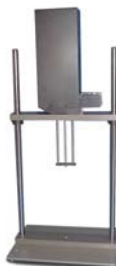
eXpert 5601 actuator mounted on a two column frame for use with a temperature chamber or larger specimens (optional).
