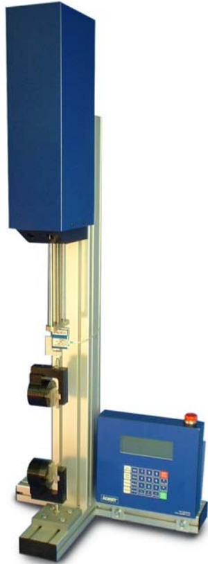
eXpert 5601 with standalone eP Digital Controller and pneumatic grips.
