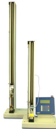
eXpert 7601 and eXpert 7601 extended frame universal testing machines with 1KN (225 Lb) capacity.
