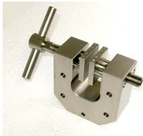
GV-20T-Ni: Temperature range -70°C - +350°C
