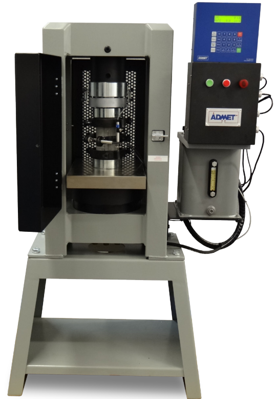
MegaForce concrete tester with Gauge Buster 2 indicator
