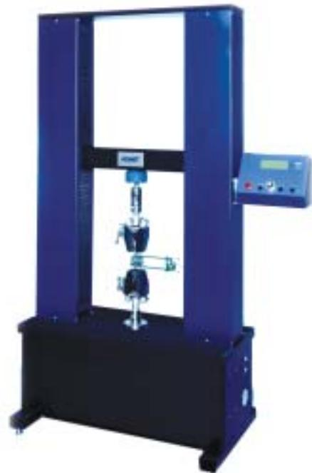
There are two classes of testing machines—electromechanical and hydraulic. *Photo: ADMET Inc.*
