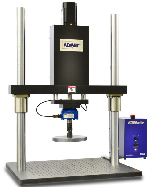
eXpert 5951 equipped to perform ASTM D3574 Constant Force Pound Test on Foam.
