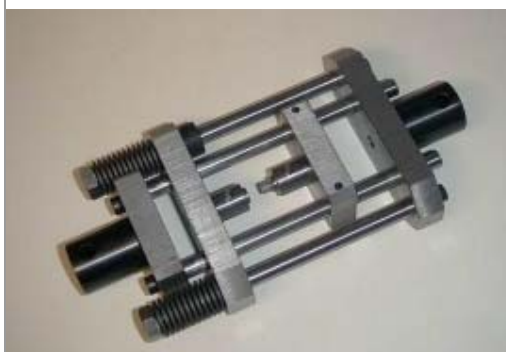
With springs to allow a slow increase in load
