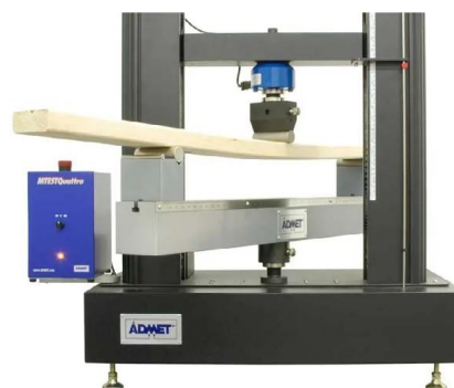
ASTM D198 Flexural Test of Lumber
