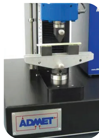
ASTM D790 Flexural Testing of Unreinforced and Reinforced Plastics
