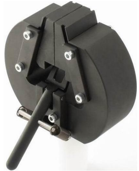
GW-10T-BP: Pyramids 1x45°, hardened steel
