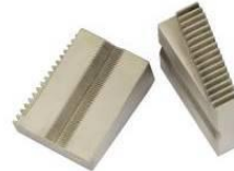
GW-T-BV -V-jaws • For all kinds of round samples • Hardened steel 58 HRC • Tooth pitch 1.2 mm
