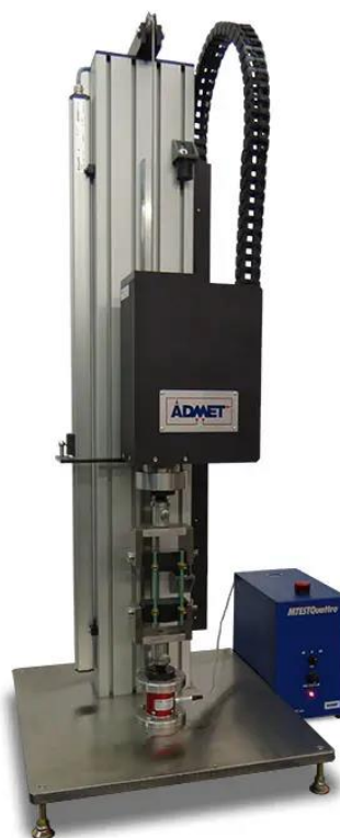
ASTM F1717 Torsion Testing of Spinal Implants
