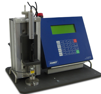
Portable 45N MicroTest for measuring stiffness of biopsy material
