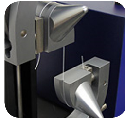
Pneumatic Grip for Suture Testing
