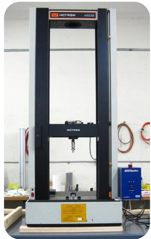
Instron 4502 (1986 – 1994) Retrofitted With MTESTQuattro® Test Controller and Software.
