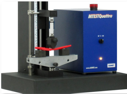
ASTM D790 three-point bend test
