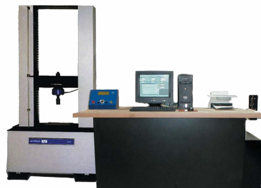
Above: Retrofit of an Instron Electromechanical UTM; Servo Hydraulic Console for Baldwin Testing Machine.
