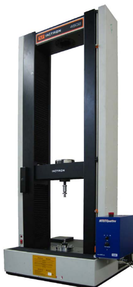
INSTRON 4502 Retrofit with new ADMET MTESTQuattro® Materials Testing System
