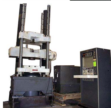
Above: Retrofit of an Instron Electromechanical UTM; Servo Hydraulic Console for Baldwin Testing Machine.
