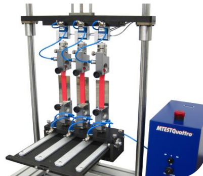
ASTM D903 Three Headed Peel Test of Adhesives
