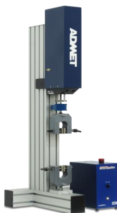
Vertically- and Horizontally-Oriented Single-Column Modular Testing Systems
